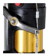
8. Attach the Creaser Cable of the ATX01TT to the main creaser cable of the Taper by inserting the hook through the S-Hook on the creaser wheel lever.
