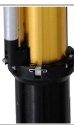
10. Hook the control tube extension to the metal pin on the control tube flange of the automatic taper.
