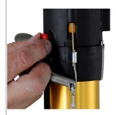
9. Tighten the red thumb screw.
