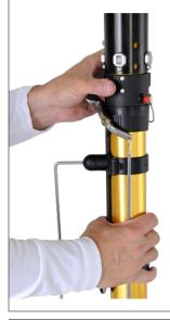
5. With your left thumb on the Alignment Fin, turn the ATX01TT to the left until it is fully seated.
