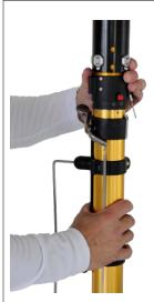
3. With the Alignment Fin in line with the center of the creaser lever, insert the internal adapter of the ATX01TT into the end of the main tube of the automatic taper.
