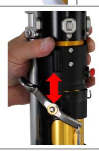
4. Make sure the Alignment Fin is in line with the center of the creaser lever before inserting the internal adapter.
