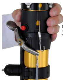
6. The red thumb screw should now be in line with the center of the creaser lever .
