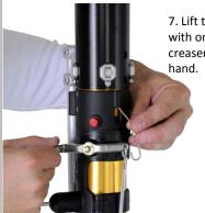
Lift the creaser wheel lever with one hand and grab the creaser hook with the other hand.
